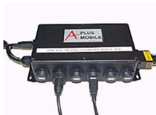
A20-HH: Harsh Environment, Power Fault Tolerant, USB 2.0 Hub with 6 Harsh USB Ports powered by A20-MC Power System
