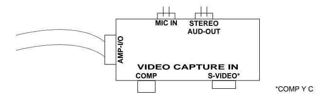
The APM-I/O connector cable will bring AUDIO-OUT, MIC-IN and other options as specified in your system configuration, such as Video Capture.
